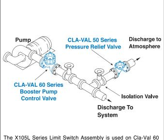
Series Booster Pump Control Valves. Flexible conduit is used for electrical connections to the solenoid control and the limit switch.
