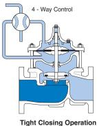
When pressure below the diaphragm is relieved and operating pressure is applied to the cover chamber, the valve closes drip-tight.
